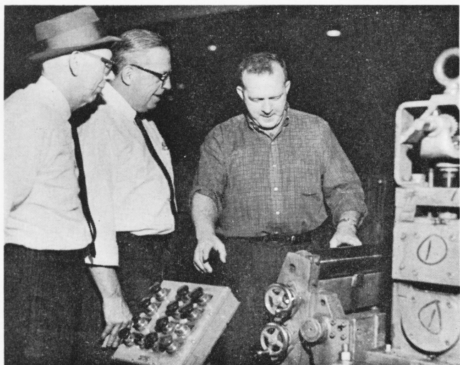
$189.00—Thomas Curtin, toolsetter in the Aluminum Mill, demonstrates to Superintendent James Hoben and Foreman Ward Hobbie the workings of the bar leveler he suggested being installed on the slitters to prevent bar jams which greatly cuts down downtime on the slitters.
